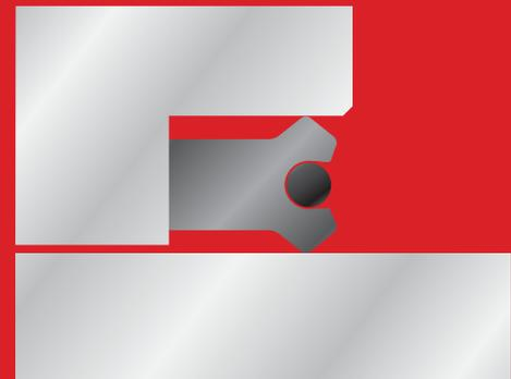
*Cutaway of an O-ring energized seals*
