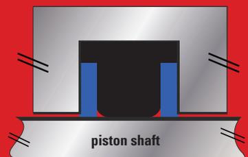
*Rod-style T-seal installed between piston shaft and barrel*
